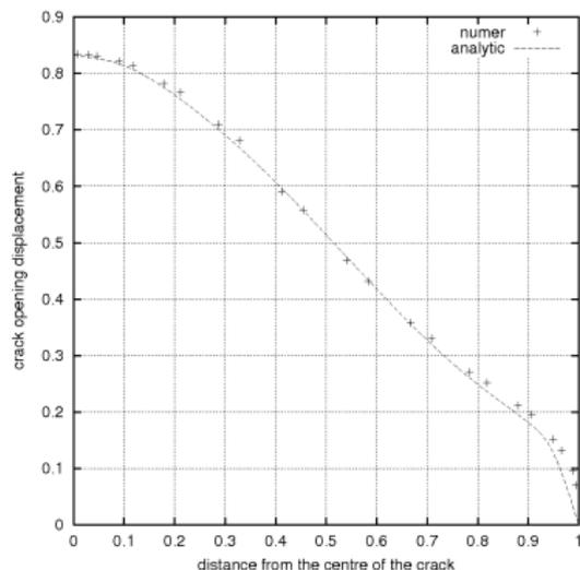
Figure: Numerical result and analytical solution ( $k_T a_0 = 3.2$ )
