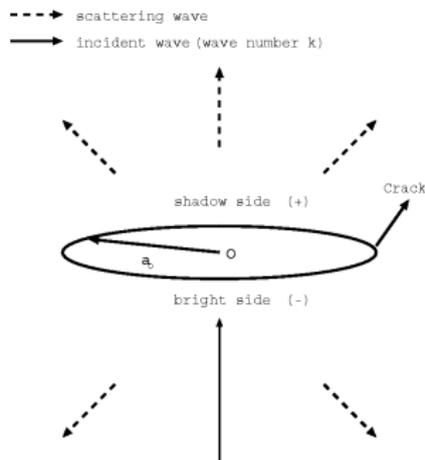
Figure: Scattering by a penny shaped crack
