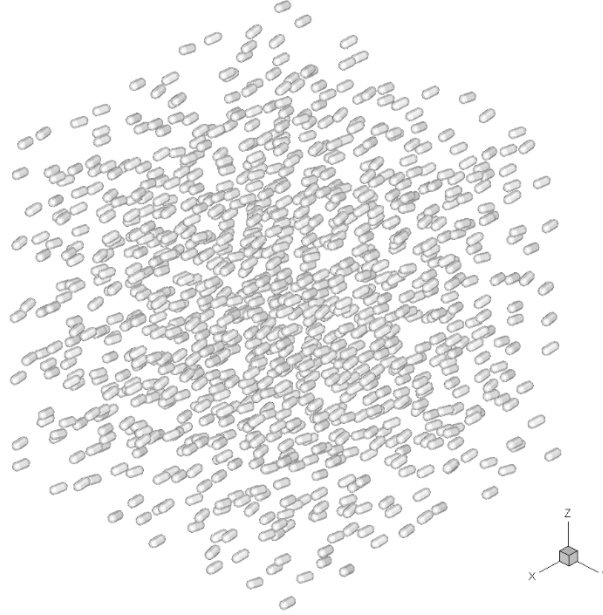
Figure 6.9. A BEM model of 1000 capsule-like scatterers with 200,000 elements.
