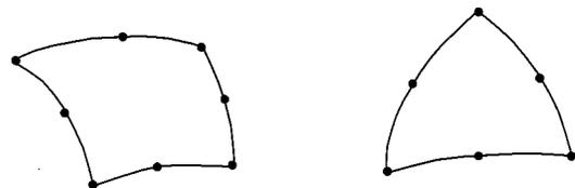
FIG. 2. Conforming quadratic boundary elements.
