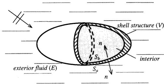
FIG. 1. A 3D shell structure immersed in fluid.
