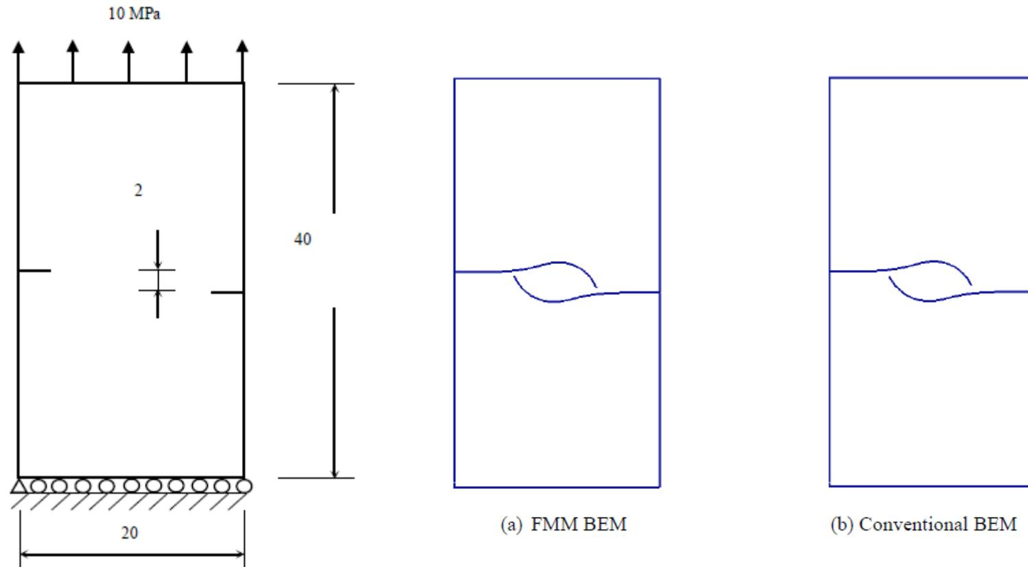
A plate with two edge cracks.
