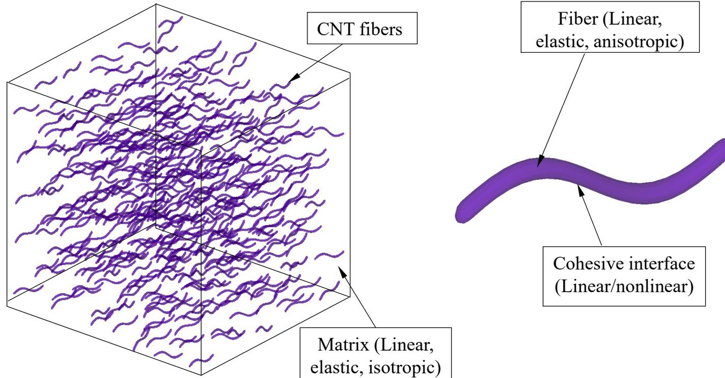
(a) An RVE with many CNT fibers (to be solved by the fast multipole BEM)
