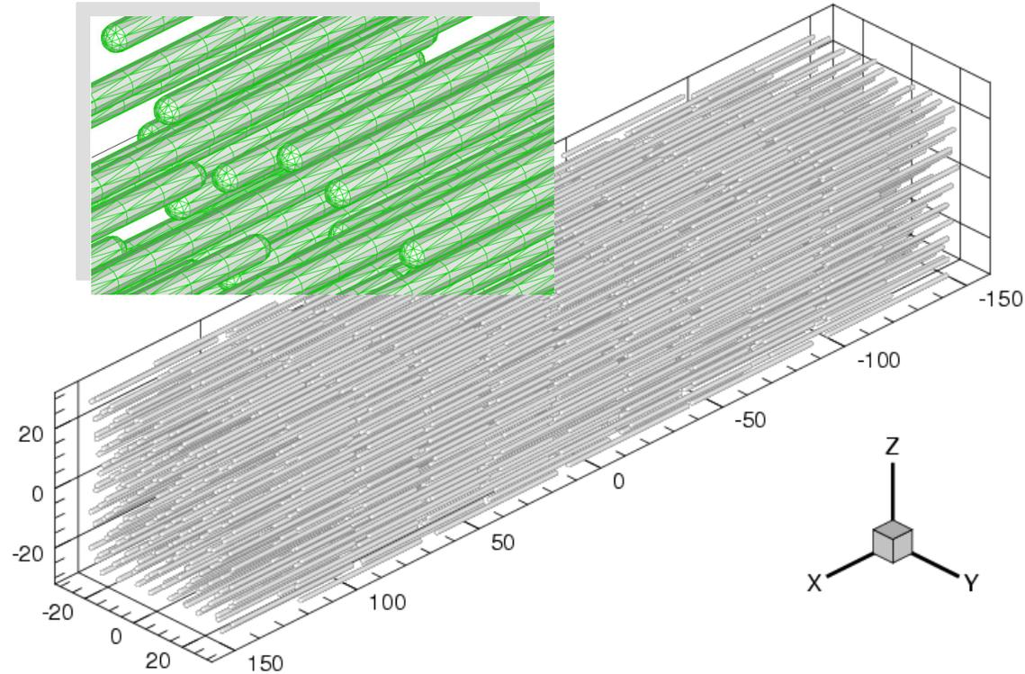
An RVE containing 2,000 CNT fibers with the total DOF = 3,612,000 (CNT length = 50 nm, volume fraction = 10.48%). A larger model with 16,000 CNT fibers (8 times of what is shown above) and **28.9M DOFs** was solved successfully on a FUJITSU HPC2500 supercomputer at Kyoto University
