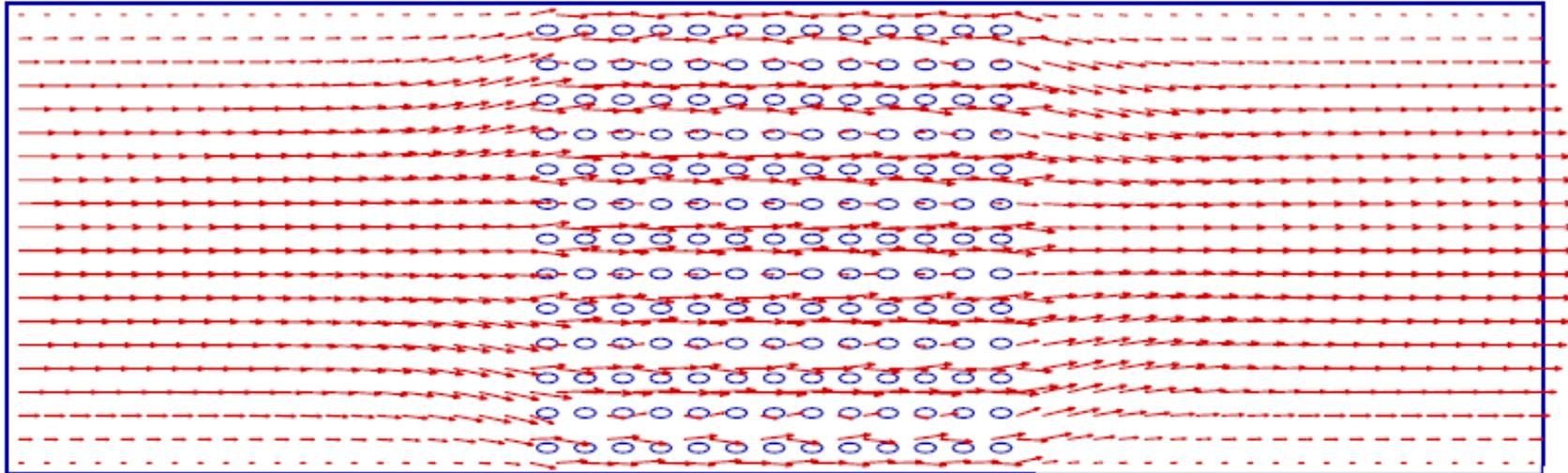
(c) A larger model with  $13 \times 13$  elliptic cylinders and  $a = 0.02h$ ,  $b = 0.5a$ , DOFs = 103,000.
