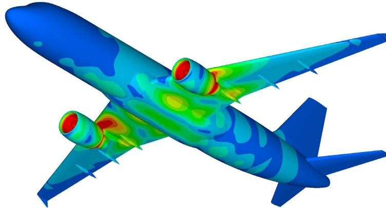
Noise propagation on the ground during the landing of an airplane, BEM model with 539,722 elements and solved with the FMM BEM in 8940 sec on a PC ( $ka = 61.5$  or  $f = 90$  Hz).
