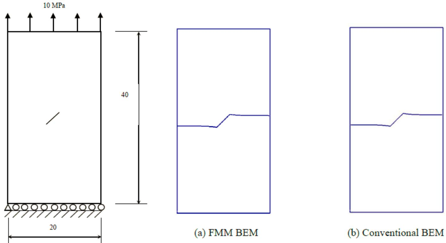
A plate with an inclined center crack.
